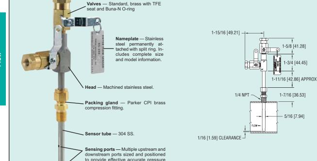
In-Line Flow Sensors are averaging Pitot tubes that provide accurate and convenient flow rate sensing for schedule 40 pipe. When purchased with a Dwyer® Capsuhelic® differential pressure gage of appropriate range, the result is a flow indicating system delivered off the shelf at an economical price.
