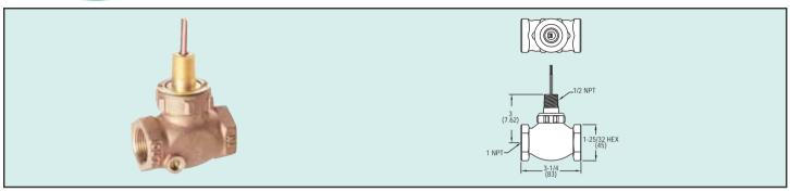
The Series GVS offers accurate flow detection with 1% repeatability and external adjustability over a broad range of flow settings. The durable construction delivers long-life reliability in either water or oil. Generous flow paths keep pressure drop low. The GVS are ideal for detection of improper flow rates in high volume lubrication, cooling or process systems.
