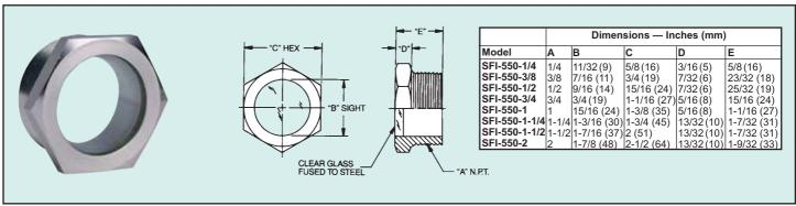
Fused glass style sight windows feature glass to metal bond for utmost reliability. Plated steel bodies have convenient hex wrench surfaces. Connections are standard NPT in sizes from 1/4" to 2". Windows are clear, ripple free, and flush with the front face, having no recess on which dirt might collect.
