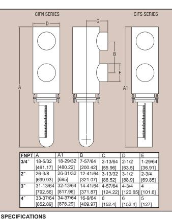
Temperature Limits: 600°F (315°C). Pressure Limits: 150 psig (10 bar).
