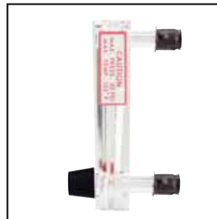
Model MMF mounts easily from front of panel. Drill two 9/32" or 5/16" dia. holes in panel on 2-1/16" centers. Insert mounting connector spuds. From rear, slide on the two spring retainers (furnished) and push on rubber or plastic tubing.
