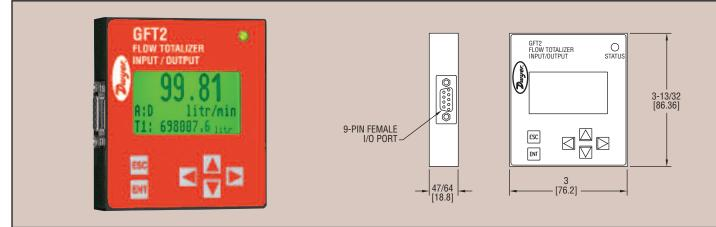
**The Series GFT2 Flow Totalizer** is a microcontroller driven device designed to linearize the flow meter and controller flow curve plus display the instantaneous flow rate, total, and accumulated total. The totalizer is intended to be used with analog flow meters and controllers with analog 0 to 5 VDC, 0 to 10 VDC, or 4 to 20 mA interface. RS-232 or RS-485 digital interface is available.
