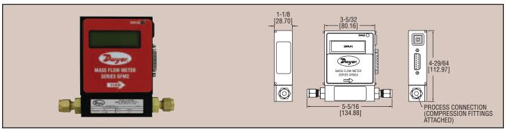
The Series GFM2 Gas Mass Flow Meter is an ideal choice for the measurement of flow rates of a wide variety of gases. GFM2 utilizes a straight tube sensor with a restrictor flow element to provide a high  $\pm 1\%$  FS accuracy and  $\pm 0.25\%$  FS repeatability.
