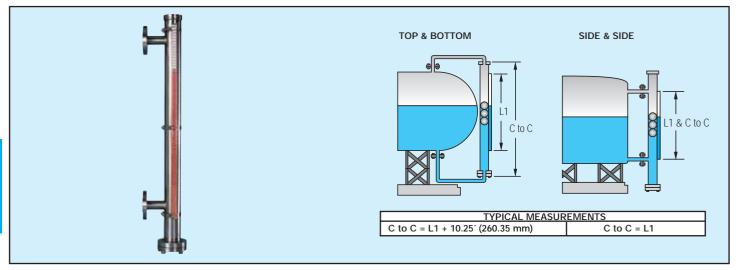
**Customize level indicators** to meet application requirements. Visi-rite level indicators are low maintenance, environmentally friendly, durable, and require no external power. Specify any indication length up to 96 inches (244 cm). View-Rite level indicators incorporate a pressure tight housing with internal float that magnetically activates external level indication flags, switches, or transmitter.
