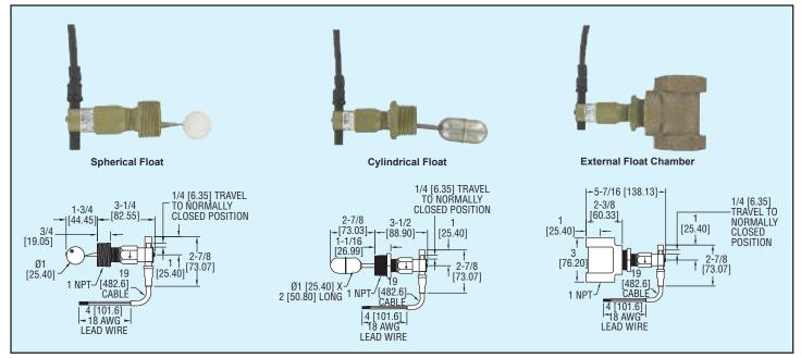
The Mini-Size Series L10 Flotect® Level Switches combine low cost with top quality materials and construction for great value and years of reliable liquid level control. Wide media compatibility is assured with a choice of brass or stainless steel bodies and external tees; polypropylene or stainless steel floats. Two basic configurations are offered; with 1" male NPT threads for direct side mounting through a half coupling or with factory installed tee for external mounting.
