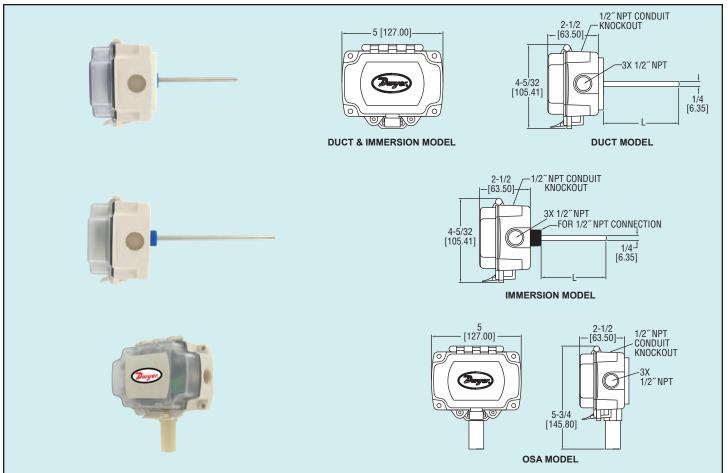
The Series WTP Wireless Temperature Sensors can be quickly installed on chilled water lines, air ducts or outside a building without having to run additional wiring. By sampling the temperature measurement every 10 seconds, the  $3.6\,\mathrm{V}$  lithium battery is able to power the unit for up to 8 years.
