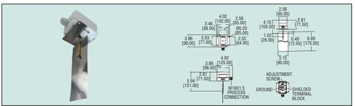
The Model AAFS-1 Adjustable Air Flow Switch is capable of detecting a wide range of air velocities with minimal user calibration. The adjustable screw changes the set point at which the SPDT snap switch engages. Quality features include a stainless steel vane, galvanized steel base, and ABS enclosure. The unit is field adjustable from 200 to 1800 FPM (1 to 9.2 m/sec).
