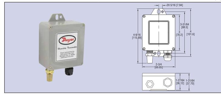
The Compact Series WHT Humidity/Temperature Transmitter is designed to withstand the elements. A removable sintered filter protects the polymer capacitance sensor from solid objects that may come in contact with the transmitter. The transmitter is available with 4 to 20 mA or 0 to 10 VDC output signals for both temperature and humidity. This transmitter is ideal for measuring outside air temperature and humidity levels for air handling economizer applications.
