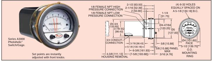
Photohelic® Switch/Gages function as versatile, highly repeatable pressure switches combined with a precise pressure gage employing the time-proven Magnehelic® gage design. The Photohelic® gage measures and controls positive, negative or differential pressures of air and compatible gases. Standard models are rated to 25 psig (1.7 bar) with options to 35 (2.4) or 80 (5.5 bar) psig. Single pressure 36000S models measure to 6000 psig (413 bar) with a 9000 psig (620 bar) rating.
